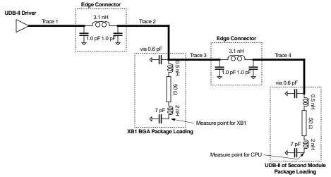
Worst Case:  $Z_0 = 60\Omega$ ,  $T_p = 180$  ps/inch, Trace 1 Length = 4.4", Trace 2 Length = 0.6", Trace 3 Length = 1.2", Trace 4 Length = 4.4"
